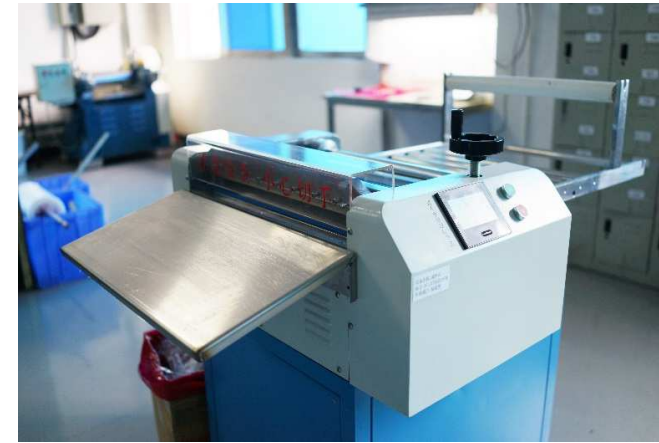
Material Cutting Machine
