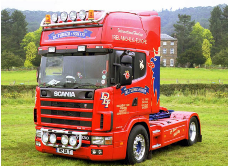
269-20. 180802. Scania 144L-530 Topline high-roof cab, 4x2 artic, 1998. R2DLT. Operator: D. L. Turner & Son Ltd, International Haulage, Underedge Farm, Rowland, Bakewell, Derbys. Location: The Peak Truck Show 2002, Bakewell, Derbys. ©BillClowes2002.
