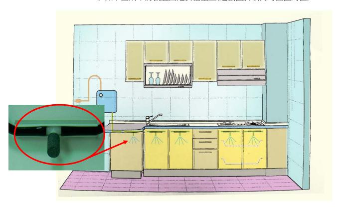
◎ CUT THE SILICON HOSE FOR DESIRE LENGTH AS PER THE CABINET INTERNAL SIZE AND THE NUMBER OF CABINET CONNECTING. INSERT THE FIRST HOSE TO THE OUTLET ON THE UNIT AND ATTACH OTHER END TO TWIN-TUBE DIFFUSER (4PCS INCLUDED), STICK THE DIFFUSER UPPER POSITION OF THE CABINET IN ORDER TO THE O₃ FLUTTER DOWNWARDS TO CIRCULATE THROUGHOUT EVERY CORNER OF THE CABINET. SINGLE-TUBE DIFFUSER (1PC INCLUDED) ONLY PACE FOR THE LAST HOSE END. 先裁切一段矽膠管,長度爲自臭氧出氣嘴到桶身內部中央,即爲預計氣泡石的位置;並接上第一個雙嘴氣泡石,此雙嘴氣
