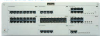
Alcatel **OmniPCX Office** allows considerable flexibility of configurations and services, thanks to its modular hardware architecture and universal back panel slots. With its unified software, Alcatel **OmniPCX Office** expands simply by adding cabinets, interface boards and MultiReflexes™.
