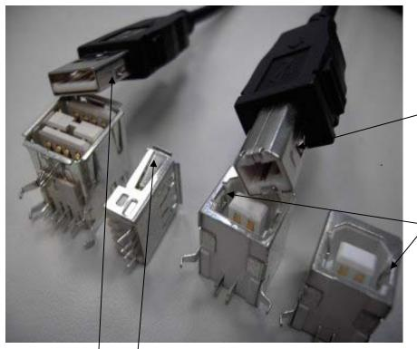
It's Locking B type Male latching at 2 side that were special designed.
