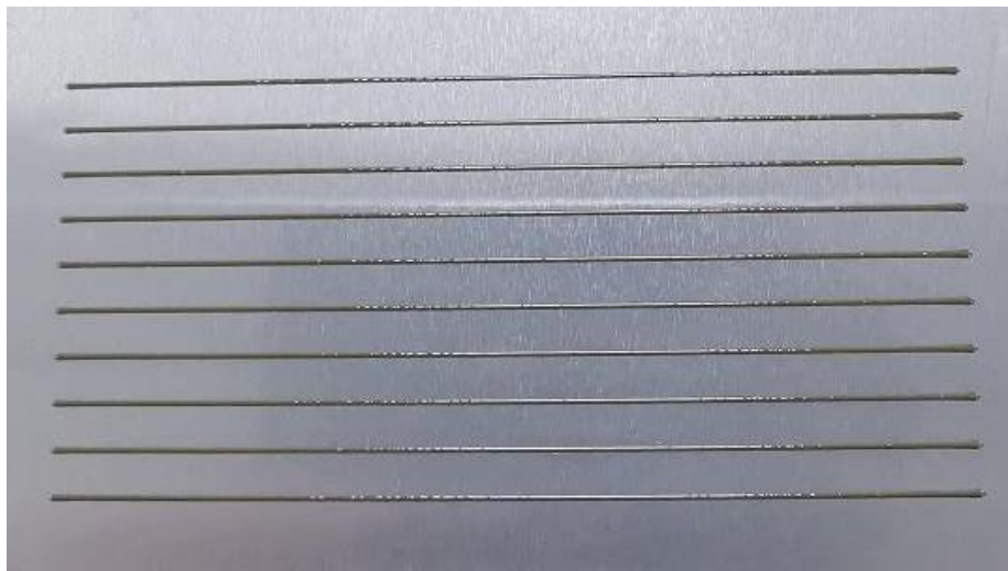
導電銀漿點膠，制程穩定0.3-0.35mm
