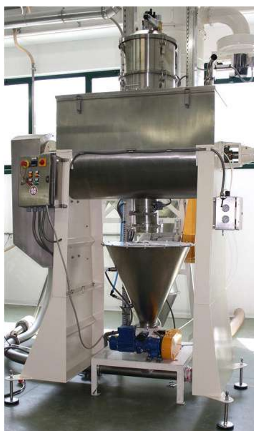
Pharmaceutical mixer working in depression.
