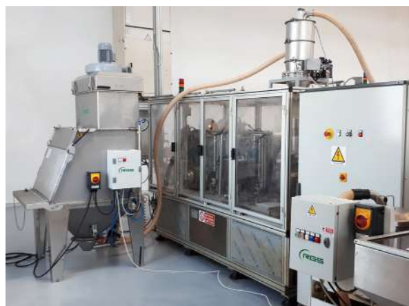
“Manual bag emptying station with cartridge filter and pneumatic vibrator”
