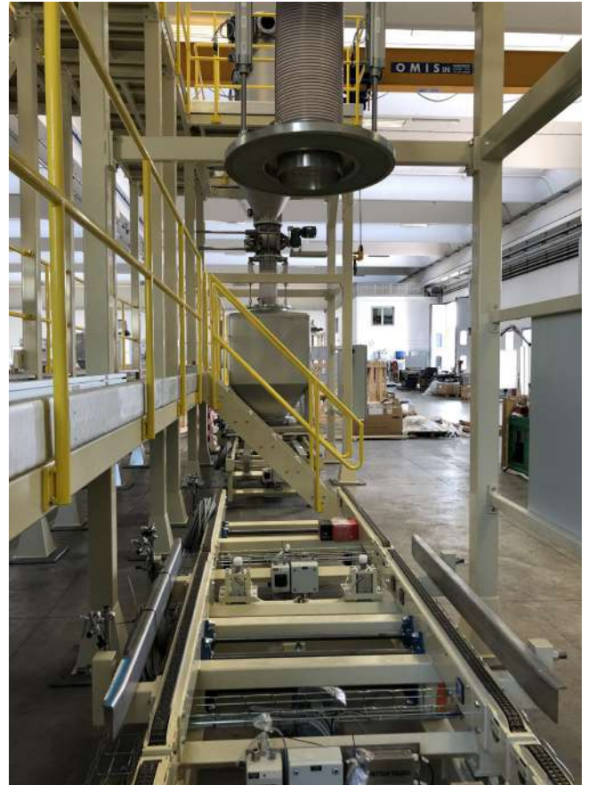
Conveyor system for tobacco powders.
