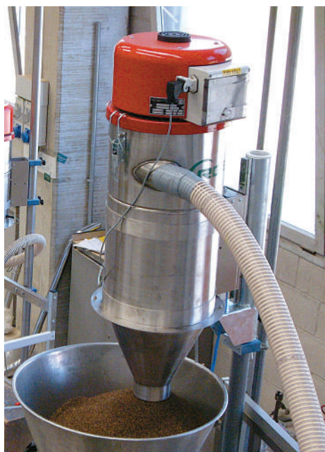
Seed conveyor system on packaging machine, made with single-phase loader equipped with anti-shutter tangential inlet.
