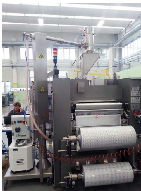
High vacuum conveyor system of pharmaceutical powders with pneumatic lifter to facilitate the positioning of the hopper over the packaging machine.
