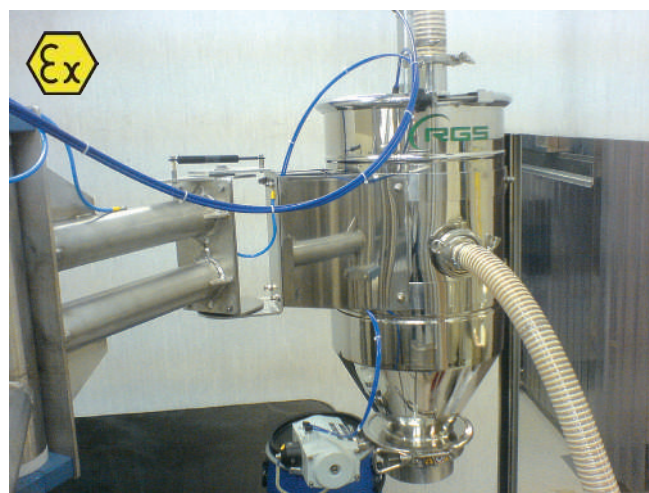
Conveyor system for mixed pharmaceutical powders made of 316L AISI stainless steel with polished finishes in a pharmaceutical industry. System realized in version ATEX for zone 21-22.
