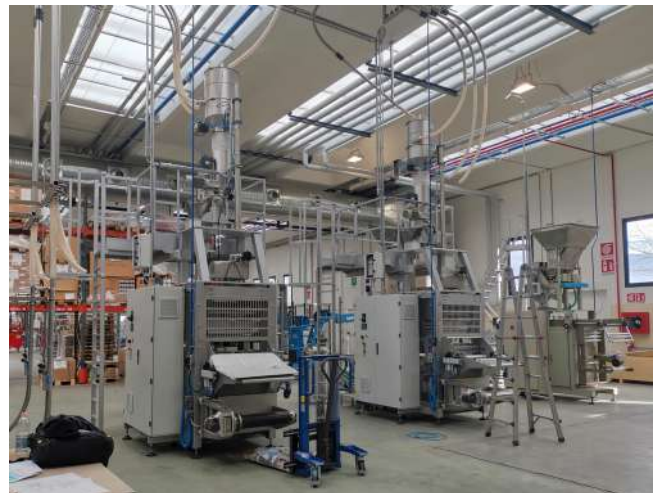
Loading system for vertical instant coffee packaging machines.
