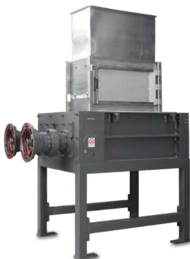
"Shredding unit suitable for all types of materials"
