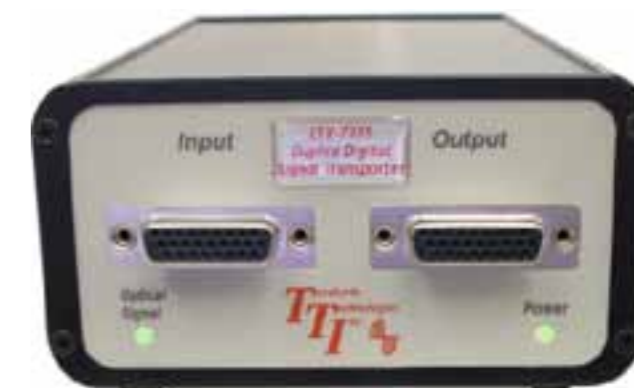
Pair a LTX-722X with a LTX-721X to configure remote high speed 12 bit A/D and D/A converter links
