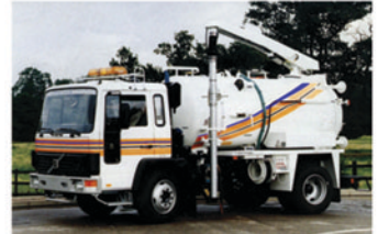
Sewer Cleaner (Jet/Vac)
